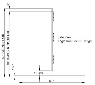
Telespar® & Angle Iron Barricades are sold in kits with three boards with your choice of sheeting. Sheeting can be on one side of the boards or both. All hardware needed for assembly is included in the kit.
