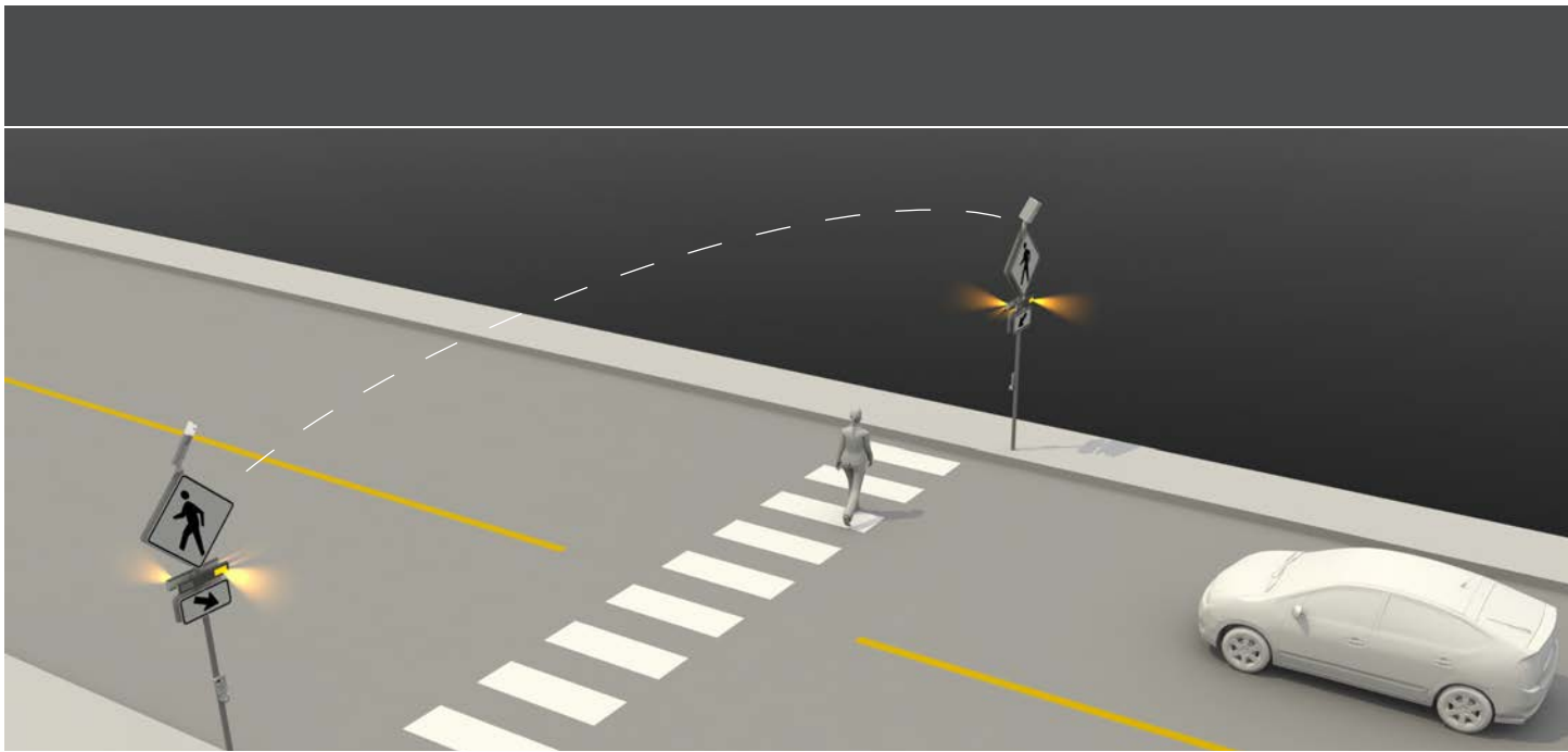
RRFBs are installed on either side of the crosswalk with a push button system that allows pedestrians to activate the beacons prior to crossing.
