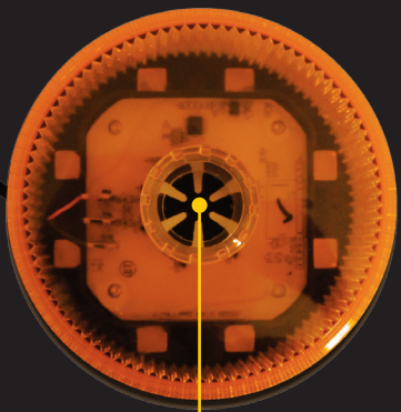
Integrated Heat Sink to control heat
