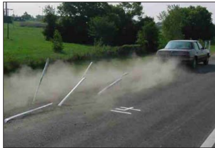
FG 500 posts are field and NTPEP tested for durability and flexibility.
