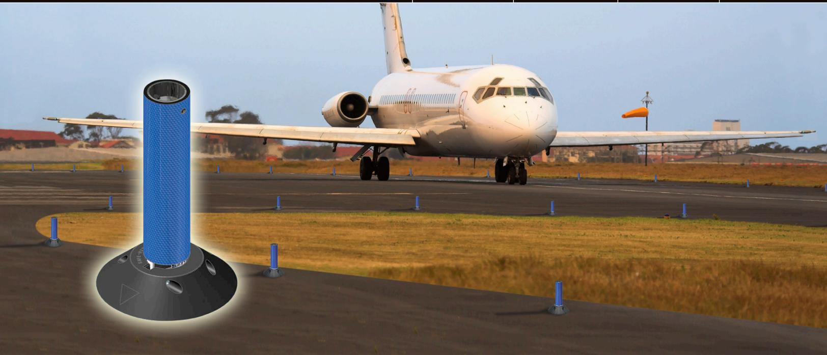
The Safe-Hit® airport marker consists of co-extruded polyethylene tube with ultraviolet inhibitors, high strength plastic fasteners and Type V retro-reflective sheeting. It has been tested and certified by ETL to the FAA's L-853 standards of the FAA Advisory Circular: 150/5345-39D. The Safe-Hit® airport marker is ideal for installations on airport taxiways, runway edges, ends and thresholds.
