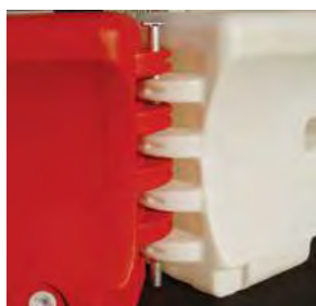
Water-Wall can pivot 30-degrees and be locked together with steel connection pins.
