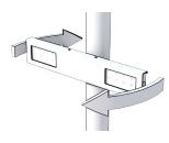
Rotate the lightbar towards the incoming vehicle lane, independent of the wire hole location.
